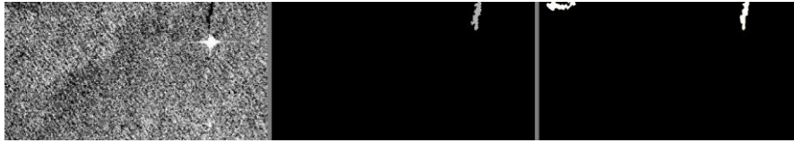
Figure 11. DL-U-net model response with median filter, SAR image, mask and response, respectively
