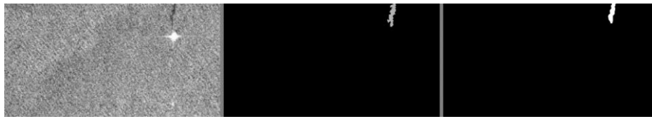
Figure 10. DL-Unet model response, SAR image, mask and response, respectively
