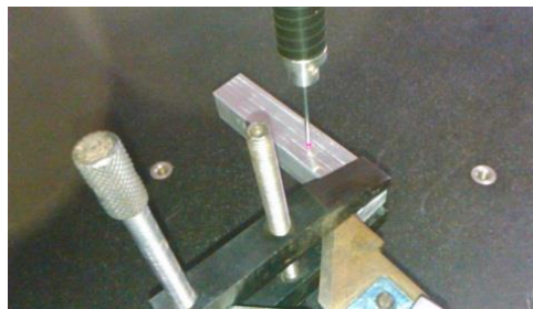
Figure 5. Flatness measurement using the coordinate measuring machine (CMM)
