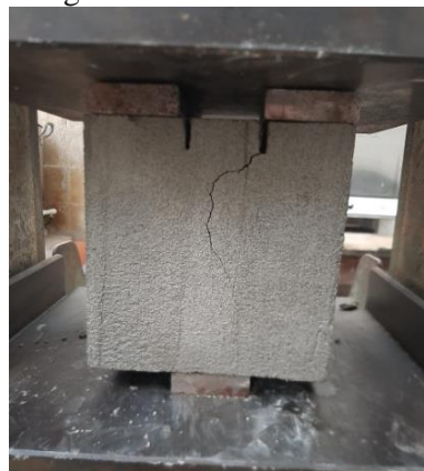
Figure 4: Failure exiting the notch.
