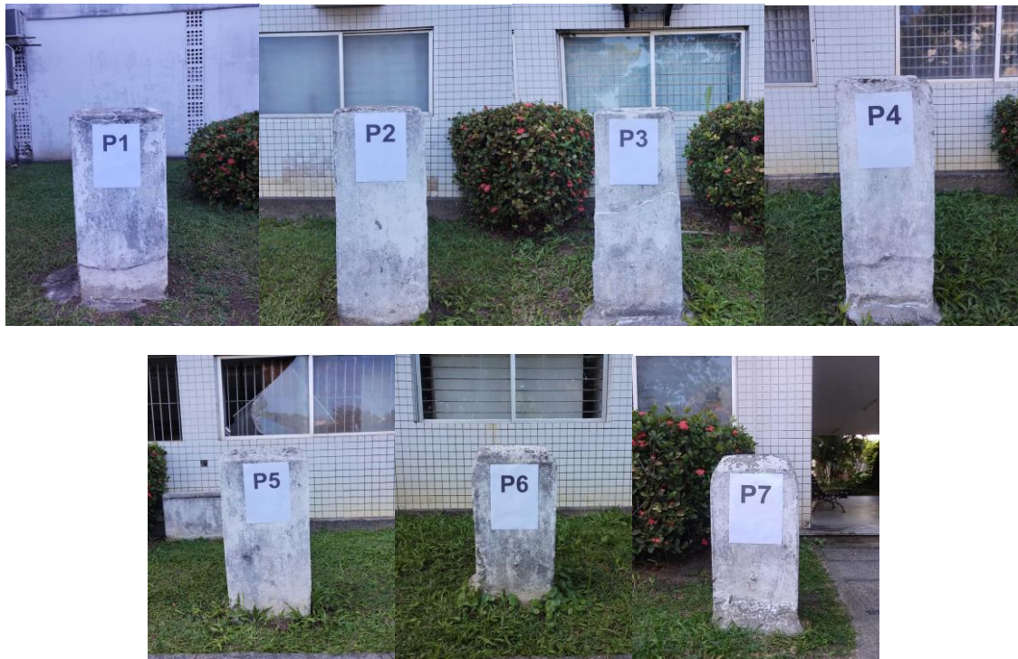
Figure 1. Each individual pillar of the EDM calibration baseline, in February 2024.
