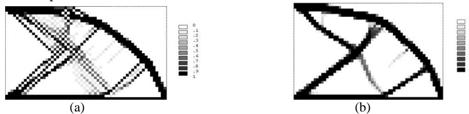
Figure 2: (a) The topology optimization result using four-node element, (b) The topology optimization result using eight-node element
