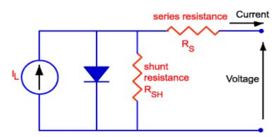
Figure 2. Equivalent circuit of PV cell representing one diode model
