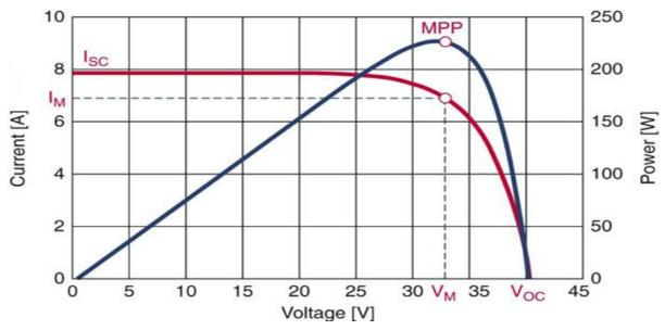
Figure 3 Graph of current and power versus voltage for a typical solar cell, showing the maximum power point and the cell's current curve.
